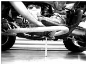
Measuring the rear frame height just in front of the foot peg.
